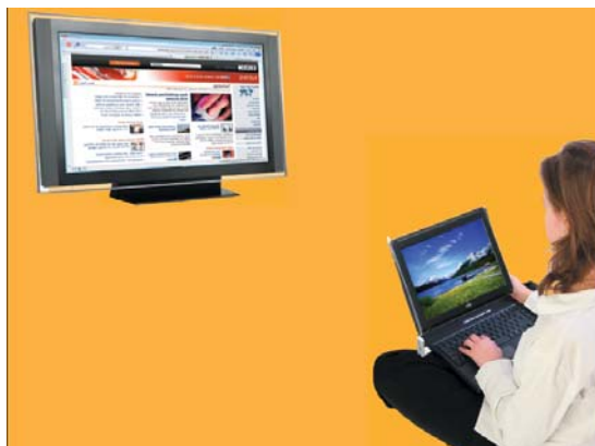
Figure 11: Extend Mode - using second display for an additional application or a movie
